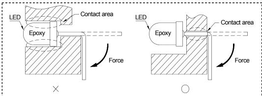
8. During soldering, component covers and holders should leave clearance to avoid placing damaging stress on the LED during soldering.
