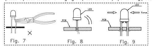
7. When bending the leads, the LED lamp should be secured by the upper part of the lead. Do not grip the epoxy lens during lead-forming bending the lead.
